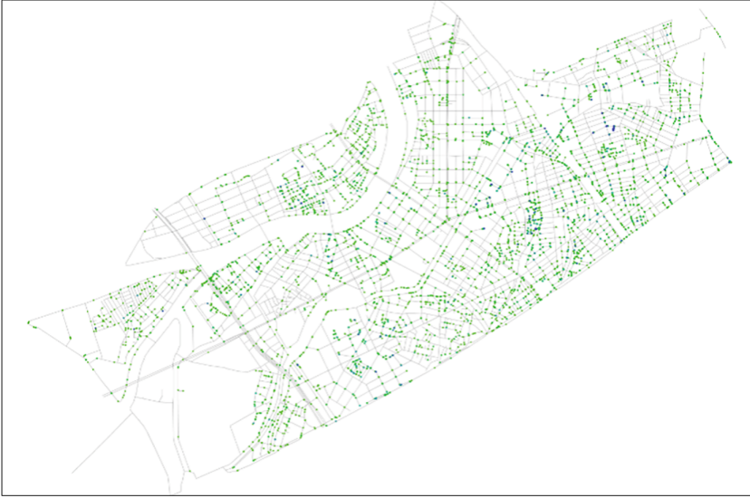
Fig. 4. Snapshot of one of the evacuation simulations conducted in this study. The lines and green points indicate roads and agents, respectively. (Color figure online)
