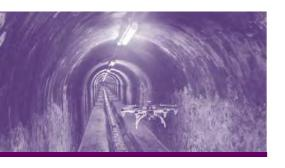
**Drones to monitor the sewer system**: ARSI has developed a micro air vehicle (MAV) to carry out autonomous inspections of the sewer network. It is a solution that bypasses the current restrictions on mobility while making the inspection process safer and
