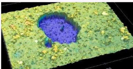
• In situ and non-destructive inspection of corrosion mechanisms and surface degradation, using surface replicas.
