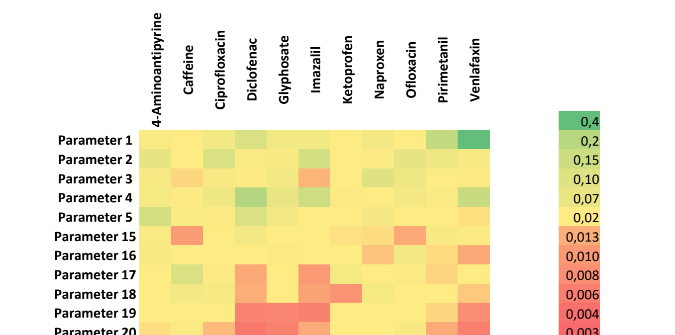
Figure 6 - Feature importance heat map of physicochemical parameters 1-5 and 15 to 20 out of the 47 that were used with the random forest model algorithm for the CECs concentration simulation.
